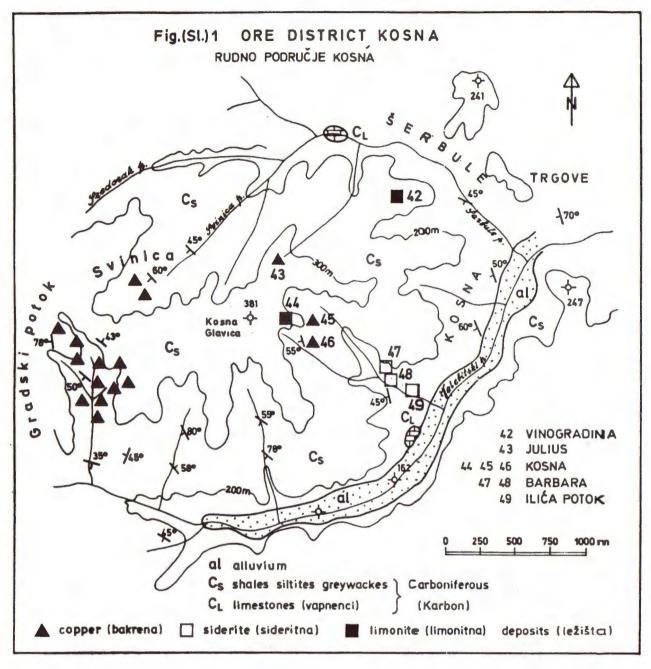
direction it forks and peters out, while, towards the west, it also quickly peters out. Its exposure extends for 25 m. The shales in which the ore was found ran NW-SE, with a dip of 50° towards NE. An adit was run from the north side of Glavice, about 10 m below the outcrop and extended for 38 m, but it traversed nothing but limonitized slates with two thin intercalations of limonite. Work was stopped because of these poor results.
