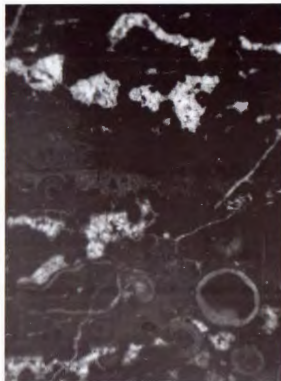
Fig. 6. Limestone with vadose features: pelletal wackestone with fenestral fabric and some vadose ooids (bottom), erosional surface and vadose ooids, chrysal silt and roof of vugs with gravitational (microstalactite) calcite cement. Tithonian of Dubrovnik environ. Facies J-1 (33x).
